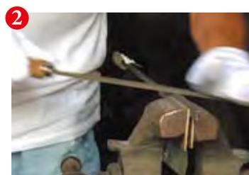
The blade is filed, and clay is applied to create the hamon temper-line patterns.
