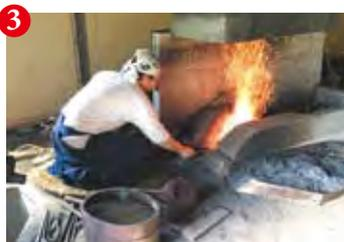
Yaki-ire (quenching) is the process in which the metal is cooled down and hardened.
